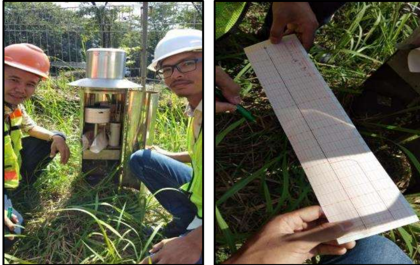
Gambar 3. Hillman Automatic Rainrecorder (A), Kertas Grafik (B)
