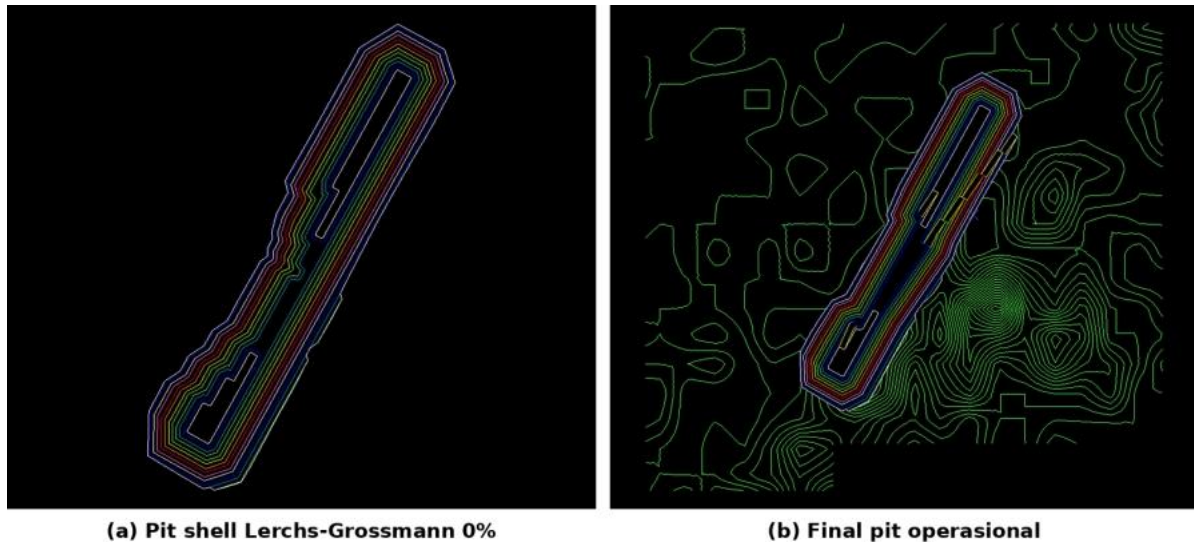
Gambar 6. Perbandingan (a) pit ramp skenario 0% dan (b) final pit operasional
